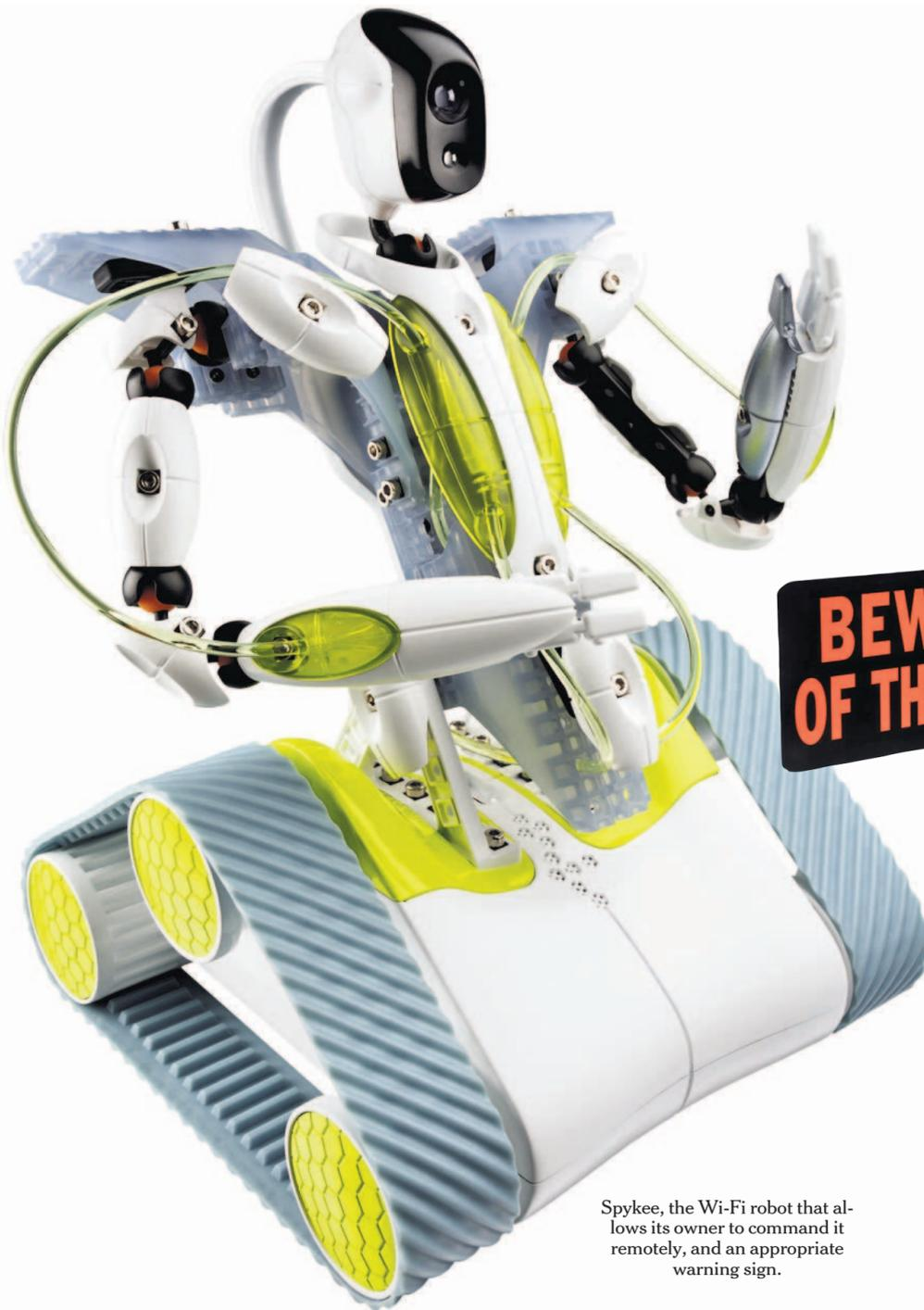
Spykee, the Wi-Fi robot that allows its owner to command it remotely, and an appropriate warning sign.
